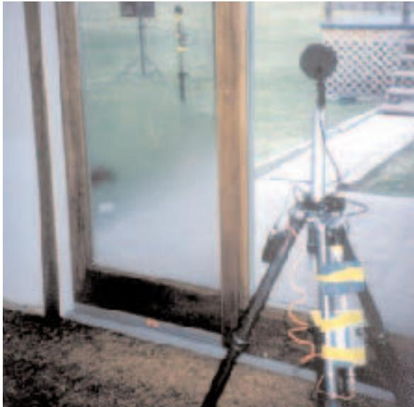
**Figure 2.** Without special glazing, frame, and sash properties, a window isn’t much more than a hole in the wall where noise will enter freely. An acoustical window, capped by a high-performance triple-track storm window, can reduce sound transmission by 50% compared to conventional windows.
